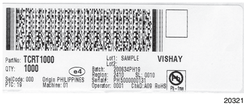
Figure 2. 2D barcode label (according to the Barcode Standard for 2D Label PDF 417) for a lead (Pb)-free device, equivalent to that shown in figure 11.
